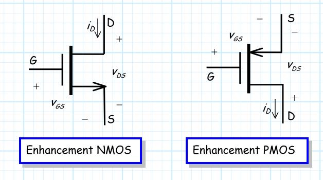
Study these symbols carefully, so you can quickly identify the symbol and the name of each terminal (e.g., source S, gate G).
